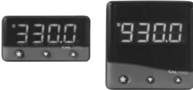
The CAL 3300 1/32 DIN and the CAL 9300 1/16 DIN miniature controllers share the same PID control strategy and features while giving the user the flexibility of a choice of panel format. Control can be optimised with a single shot autotune either on initial warm-up or at setpoint. A second setpoint can be configured in a variety of alarm modes or PID Heat-Cool strategy. A programmer offers a single ramp to setpoint with a choice of timed soak period before switching off the output.
