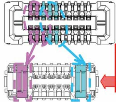
Power lines are concentrated into 2 power contacts instead of conventional multiple signal contacts.
