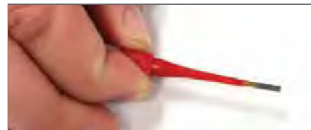
Plastic tool with contact in proper position.
