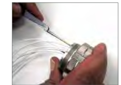
Removal of contacts with metal tool.
