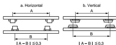
(2) If rotational error exists between two connectors, distance tolerance between the two connectors is as follows:
