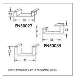
With few exceptions, the terminal block variations depicted in this catalog will readily mount in all three basic track variations. The convenience, operating flexibility and inventory reduction provided by this feature is a key element of the rail mount terminal block system.
