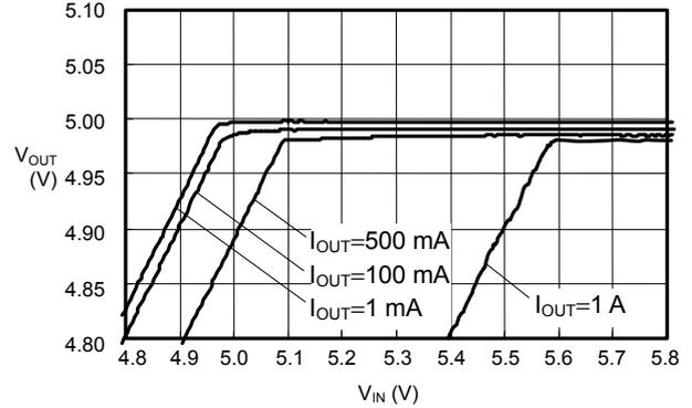
**2. Output Current ( $I_{OUT}$ ) - Output Voltage ( $V_{OUT}$ )**
