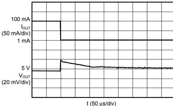
**4. ON/OFF Pin Transient Response Characteristics ( $V_{ON/OFF}=0\text{ V} \rightarrow V_{IN}$ ,  $I_{OUT}=0\text{ A}$ ,  $C_L=10\text{ }\mu\text{F}$ )**
