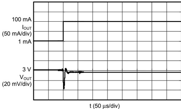
S-816A30AMC ( $V_{IN}=4\text{ V}$ )
