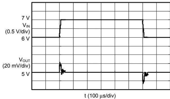
**3. Load Transient Response Characteristics (Power-on  $I_{OUT}=1\text{ mA} \leftrightarrow 100\text{ mA}$ ,  $C_L=10\text{ }\mu\text{F}$ )**
