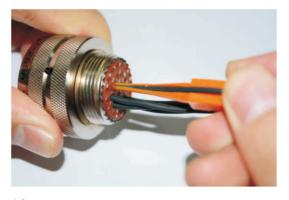
Insert tool into contact cavity until tool tip bottoms against the contact shoulder, expanding clip retaining tines.
