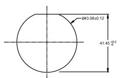
Recommended Panel Mounting Hole Recommended panel thickness: 1.6 to 4.7mm
