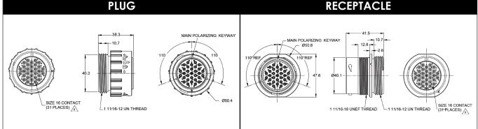
Standard and reverse terminal genders allows for custom polarization
