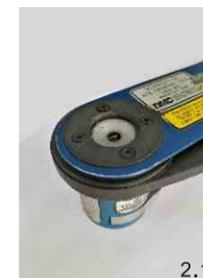
2.1 Adjust the locator of the crimp tool.
