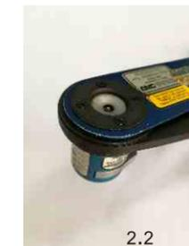
2.2 Insert the contact into the crimp tool.
