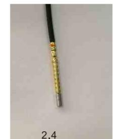
2.4 Take the wire out, check the wire is well crimped or not through the contact hole.
