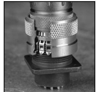
Swiftmate's coupling system uses an internal ring of formed locking fingers that glide over the threads of the receptacle. Creates a positive lock of the plug and receptacle.
