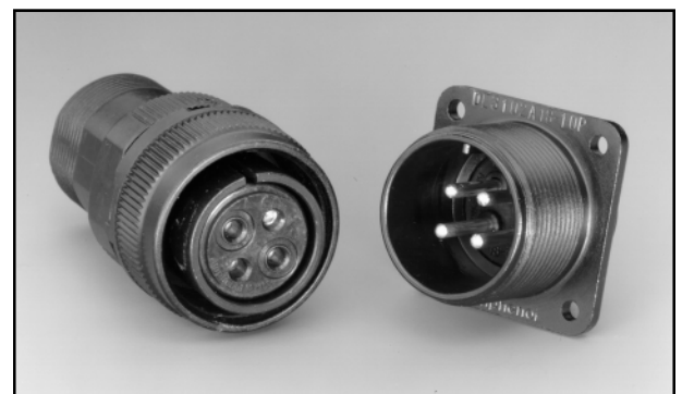
Swiftmate's coupling system uses an internal ring of formed locking fingers that glide over the threads of the receptacle. Creates a positive lock of the plug and receptacle.
