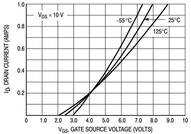
Figure 2. Transfer Characteristics
