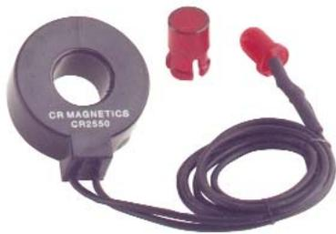
The **CR2550** Series Remote Current Indicators are designed as a low cost method for providing a visual indication of electrical current flow. The current-carrying wire is routed through the window opening in the current sensing transformer. Attached to the transformer is a high efficiency, bi-polar LED that illuminates when the current is above the turn-on point. The indicator is available as standard with an 11 inch long lead and a red, green, blue, white, amber or yellow LED indicator.
