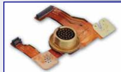
Flex Termination with MIL-C-26482 Special Connector
