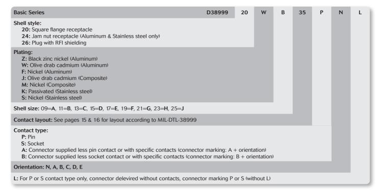
Note: To place a MIL connectors order delivered without MIL removable crimp contacts and keep P or S plus orientation marking, it must be specify clearly on the order (by adding a suffix L at the end of the P/N or specified in comment).
