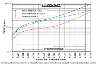
The insertion/extraction/normal force characteristics above were derived using 30 microinch gold plated con and polished steel gauge pins having a bullet-shaped tip.
