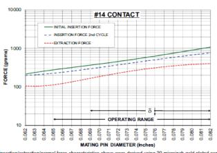
The insertion/extraction/normal force characteristics above were derived using 30 microinch gold plated contai and polished steel gauge pins having a bullet-shaped tip.
