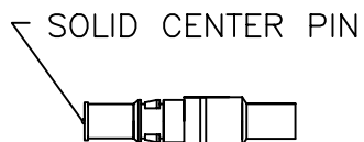
MALE COAXIAL CONTACT PART NUMBER: 682001170001
