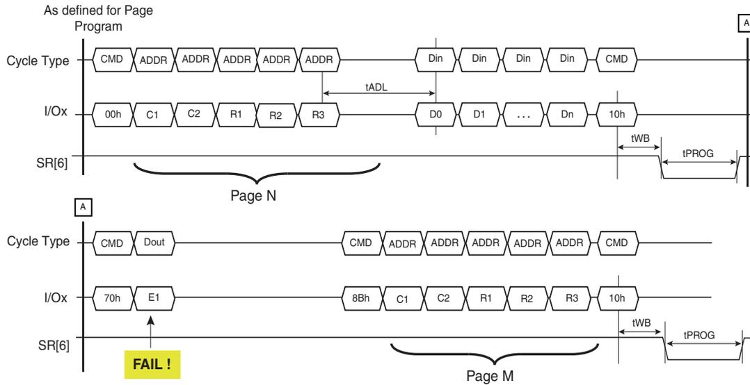
On the other hand, if the pattern bound for the target page is different from that of the previous page, data in cycles can be issued before program confirm '10h', as described in [Figure 3.2](#).
