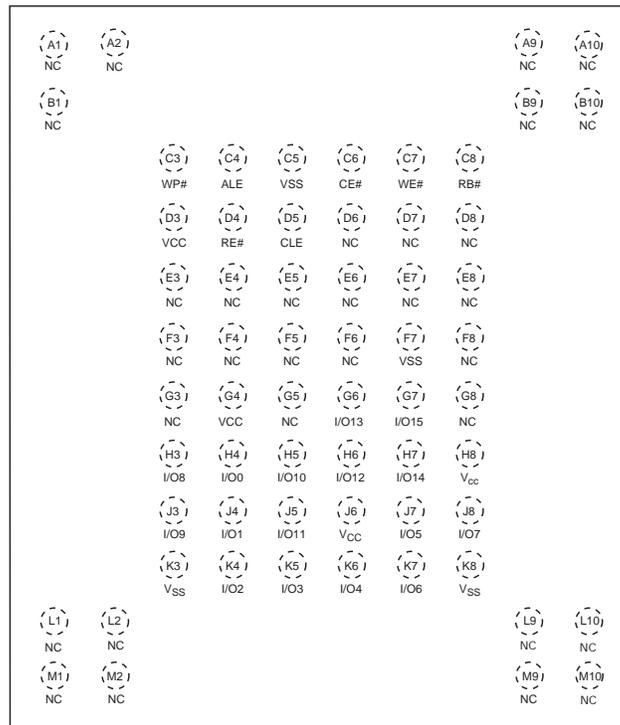
Figure 1.5 67-BGA Contact (Balls Down, Top View)
