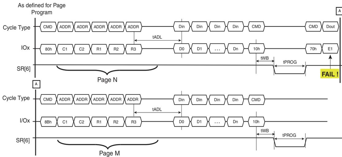
The device supports Random Data Input within a page. The column address of next data, which will be entered, may be changed to the address which follows the Random Data Input command (85h). Random Data Input may be operated multiple times regardless of how many times it is done in a page.
