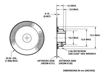
Figure 8. HEDM-5120 Codewheel/HEDM-5121 Codewheel.
