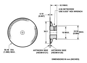
Figure 9. HEDM-6120 Codewheel/HEDM-6121 Codewheel.
