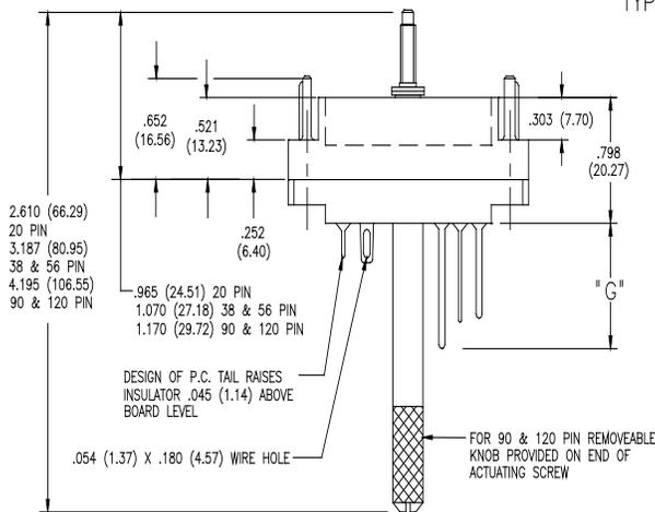
TYPICAL RECEPTACLE WITH LOCKNUT AND POLARIZING SOCKETS
