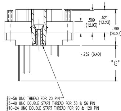
TYPICAL PLUG WITH ACTUATING SCREW, POLARIZING GUIDE PINS AND COVER
