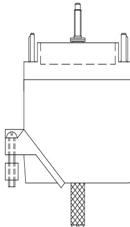
TYPICAL RECEPTACLE WITH LOCKNUT, POLARIZING SOCKETS AND COVER
