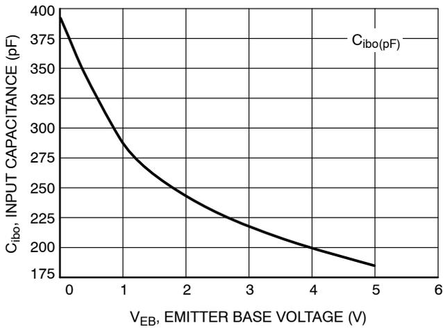
Figure 7. Input Capacitance
