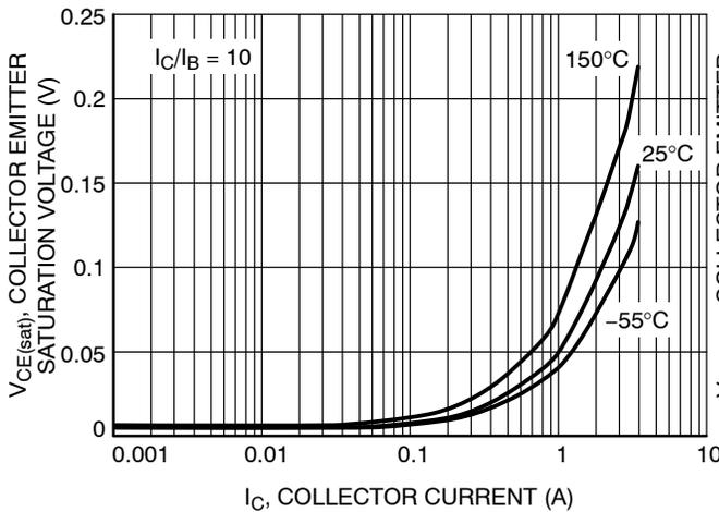
Figure 1. Collector Emitter Saturation Voltage vs. Collector Current
