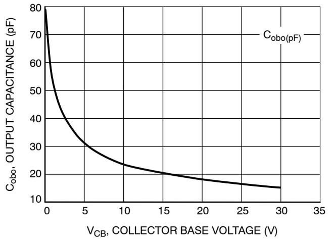
Figure 8. Output Capacitance
