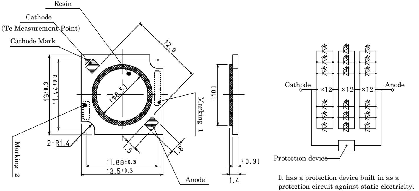
It has a protection device built in as a protection circuit against static electricity.
