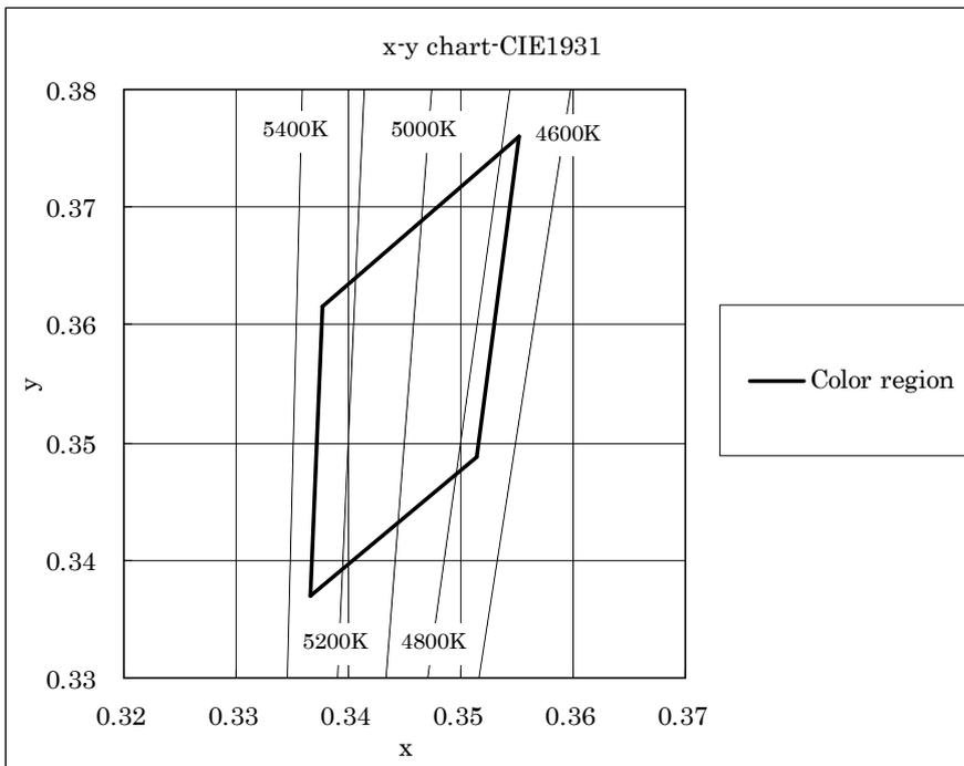
Note: The tolerance of measurement at our tester is  $V_F \pm 3\%$  ,  $\Phi_v \pm 10\%$  , Chromaticity(x,y)  $\pm 0.005$ .
