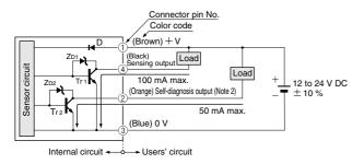
Symbols ... D: Reverse supply polarity protection diode ZD1, ZD2: Surge absorption zener diode Tr<sub>1</sub>, Tr<sub>2</sub>: NPN output transistor
