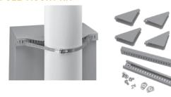
Use to mount CONCEPT<sup>TM</sup>, Networking and wall-mount enclosures to poles of various sizes and shapes. Simply attach the plated steel channel bar to the mounting holes at the back of the enclosure and wrap the stainless steel strap around the pole and through the bar. Kit includes two mounting channels, two straps suitable for 3-in. [76-mm] to 12-in. [305-mm] diameter pole and mounting hardware.
