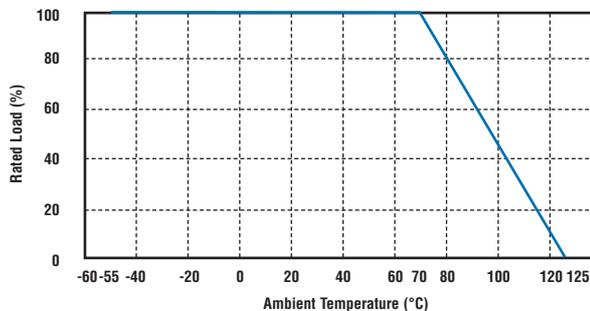
For resistors operated in ambient temperatures above 70°C, power rating must be derated in accordance with the curve.
