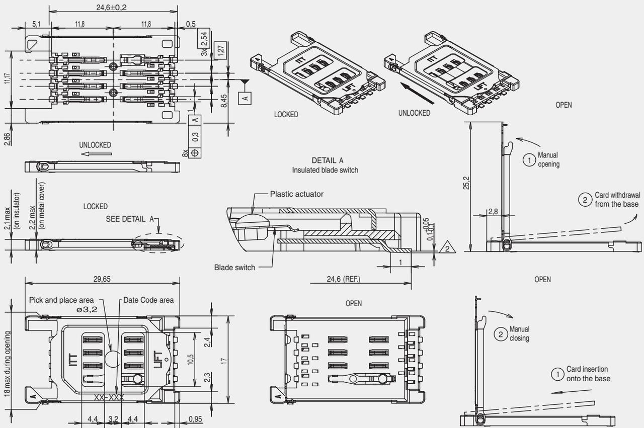
Note: Coplanarity of soldering surfaces:  $\pm 0,05$  mm
