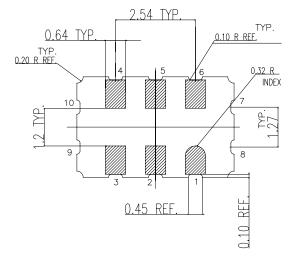
Dimensions in mm General Tolerance:  $\pm$  0.15MM Kyocera dwg ref KD-VA6432-A Package Weight ~ 0.12 grams
