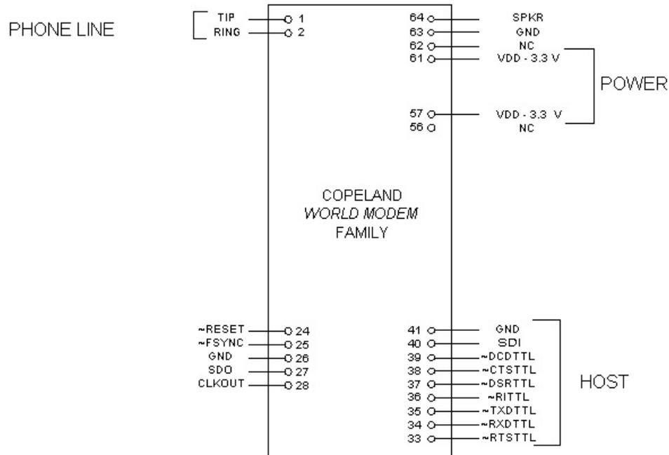
Note: Signals on pins 24,27,33-40 are TTL.
