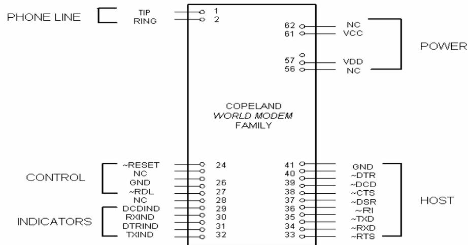
Note: Signals on pins 24,27,33-40 are TTL.
