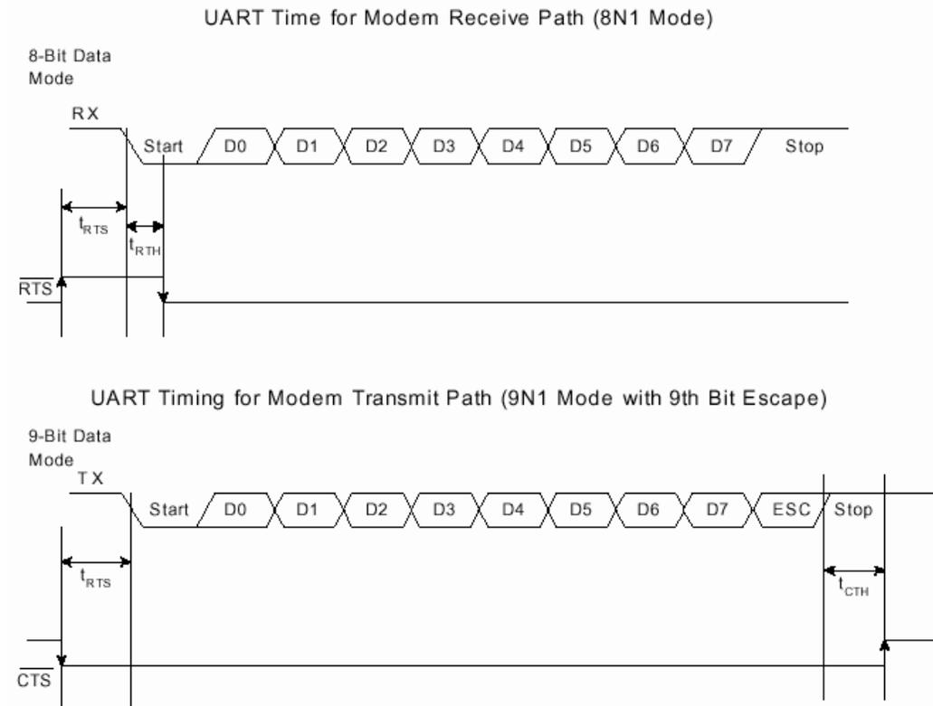
**Figure 2. Asynchronous UART Serial Interface Timing Diagram**
