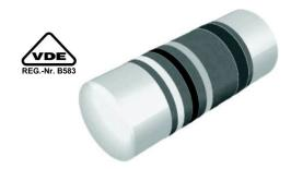
CMB 0207 speciality MELF resistors with advanced pulse load capability are the perfect choice for the protection of circuitry with signal and mains input lines from surge pulses. The resistors are also suitable for circuits exposed to high levels of electromagnetic interference or electro-static discharge. The applications are in all fields of automotive, telecommunication, industrial and medical equipment.
