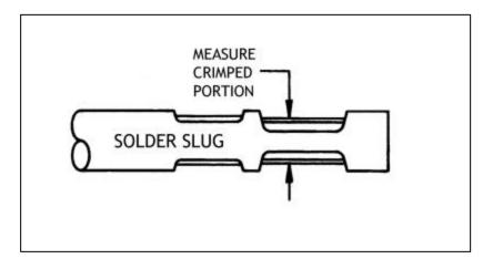
7. Insert a new solder slug after the above adjustment and repeat Steps 4 and 5 to ensure that the crimp shut height meets the dimensional specification shown on the product reel.
