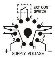
The external control switch must be a dry contact. DO NOT APPLY POWER TO PINS 5 AND 6. The external control switch can be a maximum of 10 feet away. The recommended wire is 22 gauge.
