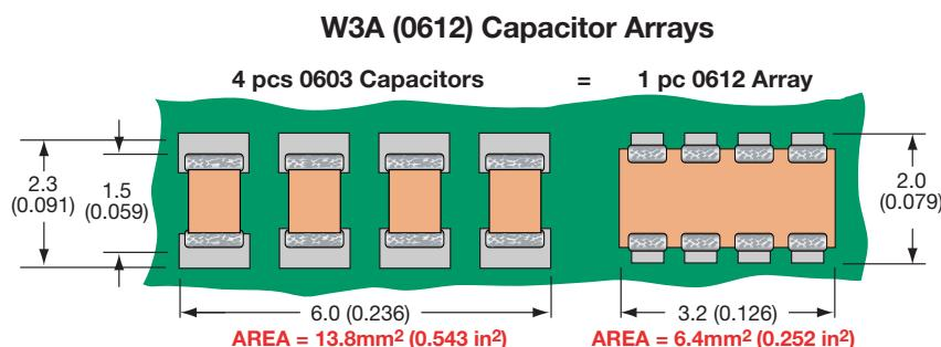
The 0612 4-element capacitor array gives a PCB space saving of over 50% vs four 0603 discretes and over 70% vs four 0805 discrete capacitors.
