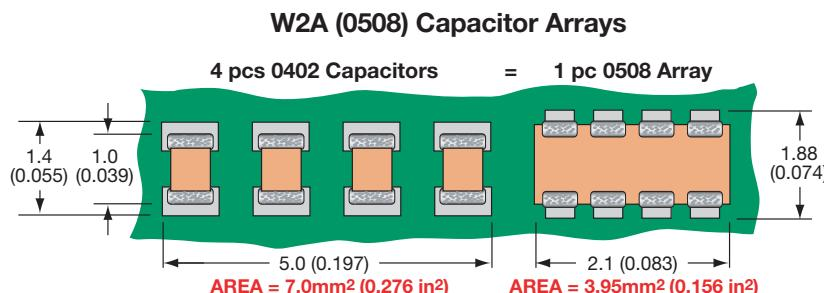
The 0508 4-element capacitor array gives a PCB space saving of over 40% vs four 0402 discretes and over 70% vs four 0603 discrete capacitors.
