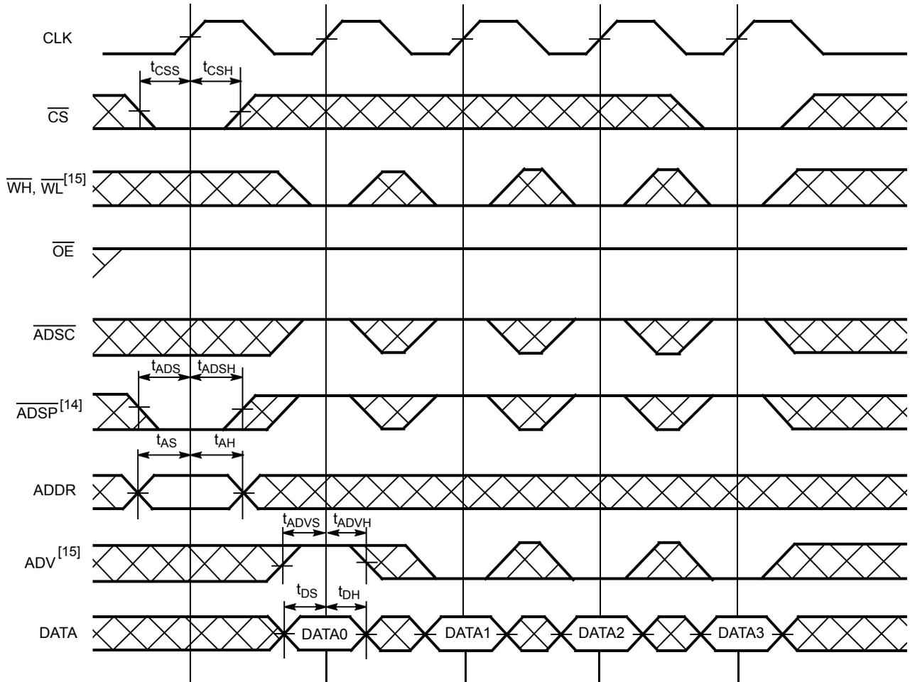
**Output Timing (Controlled by  $\overline{\text{CS}}$ )**
