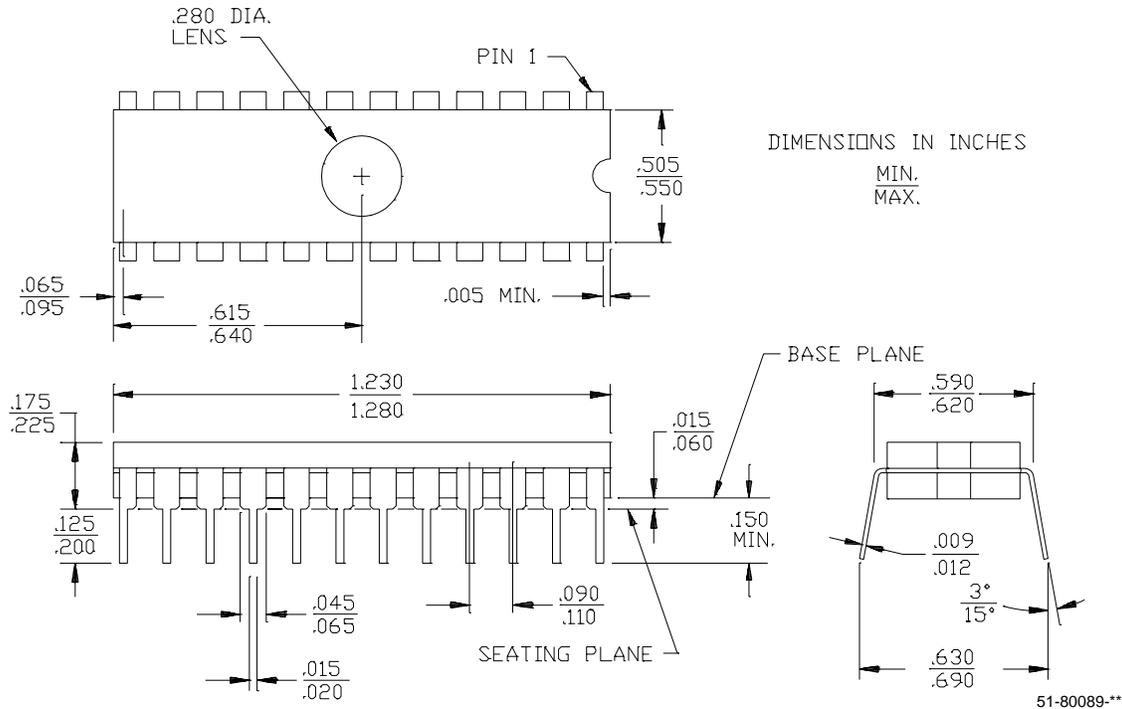
**24-Lead (300-Mil) Windowed CerDIP W14**
