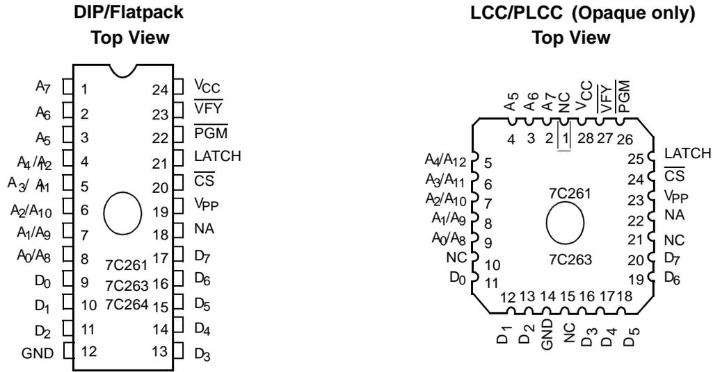
**Figure 1. Programming Pinouts**
