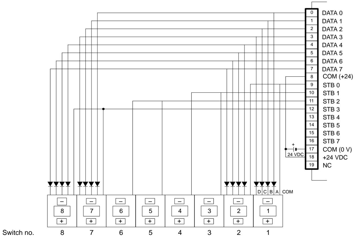
The table below shows the combinations made possible when the digital switches are wired as shown in the figure above.
