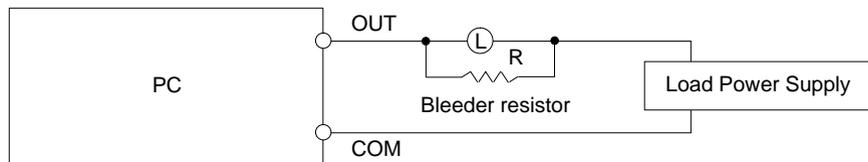
Determine the value and rating for the bleeder resistor using the following formula.
