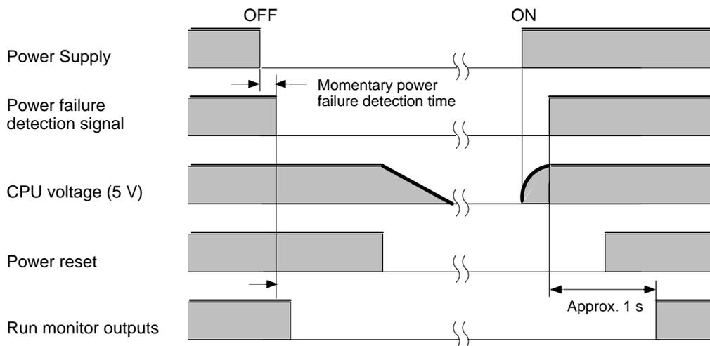
The PC ignores all momentary power failures if the interruption lasts no longer than 10 ms. If the interruption lasts between 10 and 25 ms, the interruption may or may not be detected. If the supply voltage drops below 85% of the rated voltage for longer than 25 ms (less for the DC Power Supply), the PC will stop operating and the external outputs will be automatically turned OFF. Operation is resumed automatically when the voltage is restored to more than 85% of the rated value.
