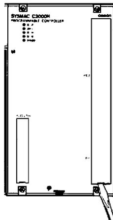
Use a standard screwdriver to remove the Memory Pack compartment cover.
