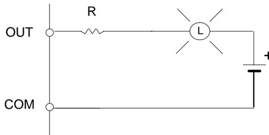
**Transistor Output Residual Voltage**
