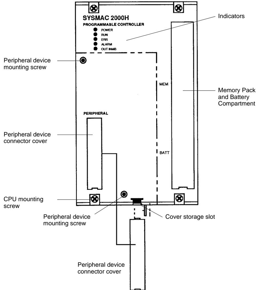
**Peripheral Device Connector** The CPU is equipped with one connector for peripheral devices. A peripheral device, such as the CPU-Mounting Programming Console, can be mounted directly to the CPU and does not require a connecting cable. To mount the CPU-Mounting Programming Console or any other peripheral device directly to the CPU, follow these steps:
