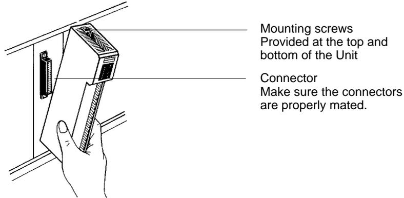
The figure below shows one I/O Unit mounted directly to the left slot of the CPU Rack.
