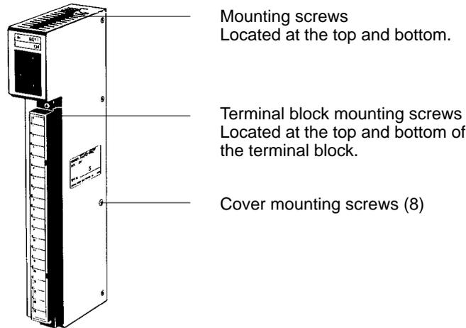
3. Remove the screws that mount the Output Unit to the Backplane. Pulling the Unit toward you remove the Output Unit from the Backplane.
