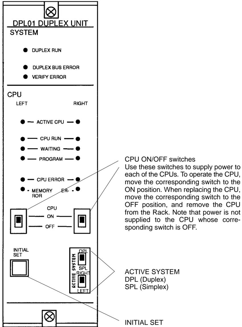
3. Next, select the active CPU by setting the Active Switch to RIGHT or LEFT. In the example above, the right CPU is the active CPU.
