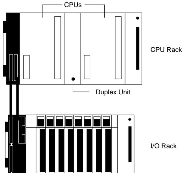
While the Duplex System is in operation, one of the two CPUs has "active" status and the other CPU has "standby" status. The active CPU executes the program and controls the I/O Units while the standby CPU merely executes the program, but does not control the I/O Units. The status of the CPUs can be determined by setting the selector switch on the front panel of the Duplex Unit.
