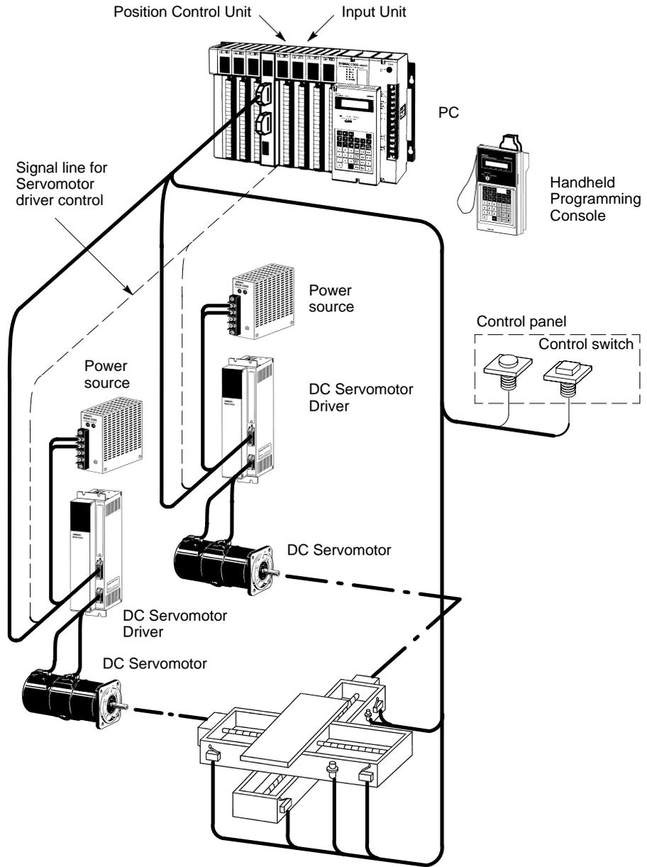
In the typical Control System example shown above, a PC controls the movement of the workpiece bed across two horizontal axes using Limit Switches and Servomotors to monitor and control movement.
