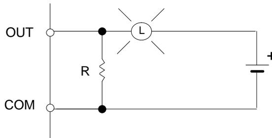
Another way of protecting the Output Unit lets the load draw a small current (about one third the rated current) while the output is OFF, significantly reducing the surge current. This circuit (shown below) not only reduces the surge current, but also reduces the voltage across the load at the same time.
