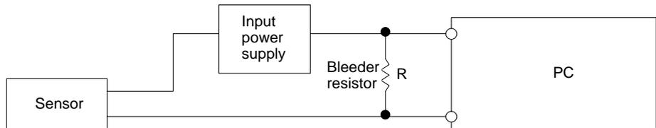
If the leakage current is less than 1.3 mA, there should be no problem. If the leakage current is greater than 1.3 mA, determine the value and rating for the bleeder resistor using the following formulas.
