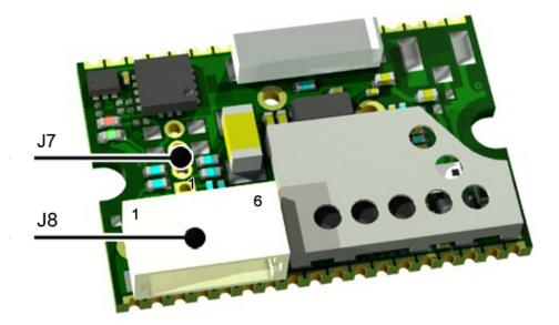
Figure 7: 4x1 through holes row J7 and the JST connector J8 mounted on the component side of the PCB.
