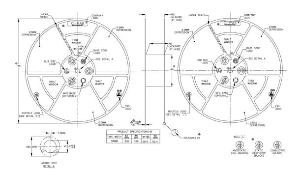
Figure 18: Tape reel dimensions.
