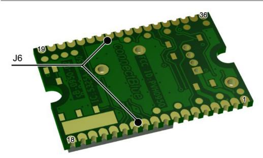
Figure 6: The solder pads J6 are available on the long edges of the bottom side of the PCB.
