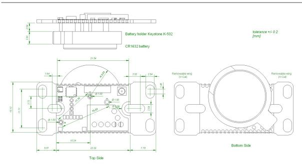
Figure 12: cB-OLP425 dimensions with mounting wings (optional, on request only) and CR1632 battery holder.
