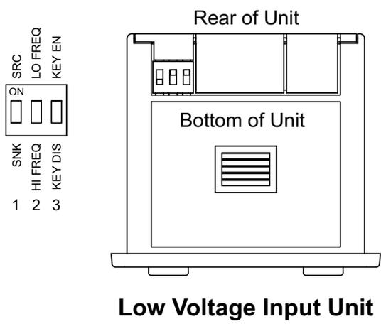
Low voltage input units have 3 DIP switches that must be positioned appropriately prior to wiring.
