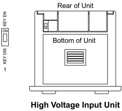
High voltage input units have 1 DIP switch to enable or disable the front bezel keypad.
