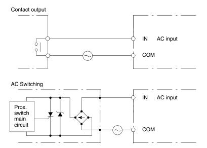
**Note** If a reed switch is used as the input contact of the AC Input Unit, the reed switch must have a permissible current capacity of 1 A minimum, otherwise contact weld may result due to inrush current.
