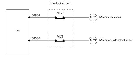
This circuit prevents outputs MC1 and MC2 from both being ON at the same time. Even if the PC is programmed improperly or malfunctions, the motor is protected.
