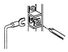
Use ring crimp terminals for wiring. Do not connect bare stranded wires directly to terminal blocks.
