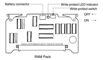
To write data to the RAM Pack, move the write-protect switch to the OFF position. After data is written to the RAM Pack, be sure to move the write-protect switch to the ON position to protect the data from further alterations. If you try to write data to the Memory Pack while the write-protect switch is in the ON position, the message DISABLED ROM will appear on the Programming Console.
