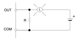
Another way of protecting the Output Unit lets the load draw a small current (about one third the rated current) while the output is OFF, significantly reducing the surge current. This circuit (shown below) not only reduces the surge current, but also reduces the voltage across the load at the same time.
