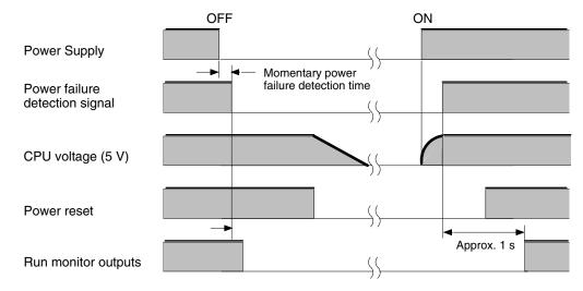
The PC ignores all momentary power failures if the interruption lasts no longer than 10 ms. If the interruption lasts between 10 and 25 ms, the interruption may or may not be detected. If the supply voltage drops below 85% of the rated voltage for longer that 25 ms (less for the DC Power Supply), the PC will stop operating and the external outputs will be automatically turned OFF. Operation is resumed automatically when the voltage is restored to more than 85% of the rated value.
