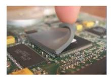
CoolZorb 400 is a hybrid absorber/thermal management material that is used for EMI mitigation. Product is used like a traditional thermal interface material between heat source such as an IC and heat sink or other heat transfer device or metal chassis. CoolZorb 400 also functions to suppress unwanted energy coupling, resonances or surface currents causing board level EMI issues.
