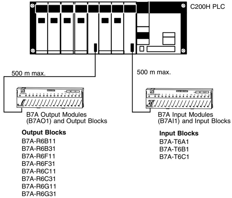
**Note** C200H-B7AI1/B7AO1 units cannot connect to a high speed B7A link terminal with transmission delay time of 3 m sec.
