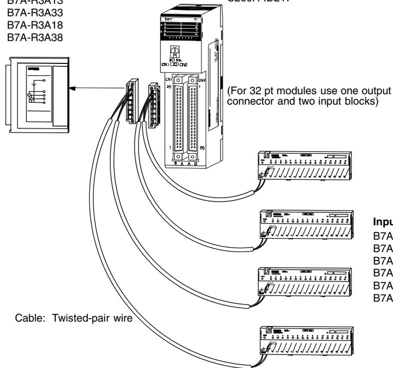
(For 32 pt modules use one output connector and two input blocks)
