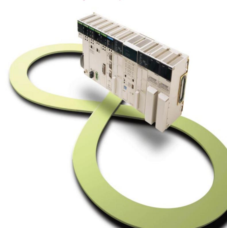
CVM1D Programmable Controllers inherit the advantages from the CV/CVM1 Series and go a step further by incorporating double systems for higher reliability. These PCs are available as a simplex system with double Power Supply Units or as a duplex system with double Power Supply Units and CPU Units. Duplex systems offer even higher reliability than conventional CV/CVM1-series systems.
