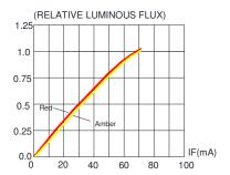
FIG.2 RELATIVE LUMINOUS FLUX VS. FORWARD CURRENT
