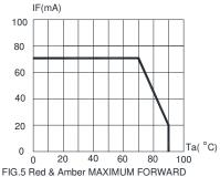
IG.5 Red & Amber MAXIMUM FORWARD DC CURRENT VS AMBIENT TEMPERATURE (Tjmax=110°C)
