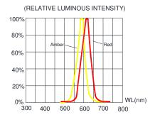
FIG.4 RELATIVE LUMINOUS INTENSITY VS. WAVELENGTH.
