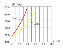
FIG.1 FORWARD CURRENT VS. FORWARD VOLTAGE.
