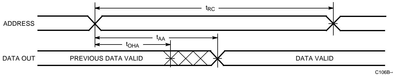
**Read Cycle No. 2 ( $\overline{OE}$  Controlled)<sup>[12, 13]</sup>**
