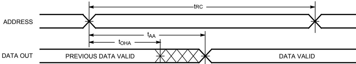
Figure 5. Read Cycle No. 2 ( $\overline{OE}$  Controlled) [12, 13]
