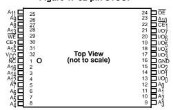
Figure 2. 32-pin TSOP I [1]
