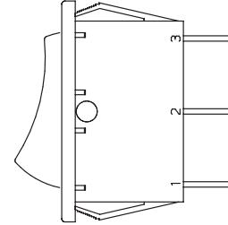
**NOTE:** Orientation of actuator marking and terminals.
