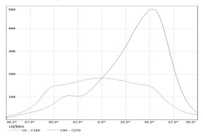
Luminaire: Ledil Oy C12049\_STRADA-FT (Luxeon T 71lm @ 250mA) Efficiency=92% Lamps: 1 x Luxeon T 71lm @ 250mA (LXH8-FW30-3) CCT=3158K P=0,75W I=250mA
