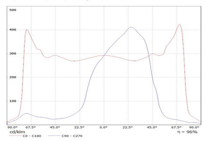
Luminaire: LEDiL Oy C13140\_STRADA-T-6X1-DWC\_(SQ-PC) Eff.95.8% Lamps: 1 x Osram Square PC (586.106lm@250mA)
