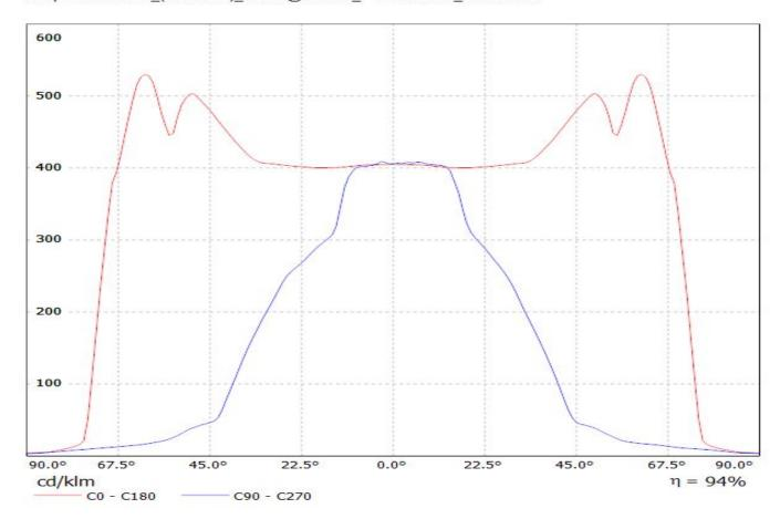
Luminaire: LEDiL Oy C14128\_TATIANA-1X4-B\_(XM-L2) Lamps: 1 x XM-L2\_(TATIANA)\_357Im@250mA\_P=2.84023W\_I=249.8mA
