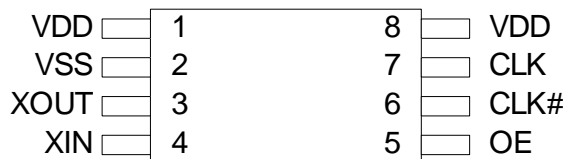
Figure 1. Pin Diagram - 8-Pin TSSOP
